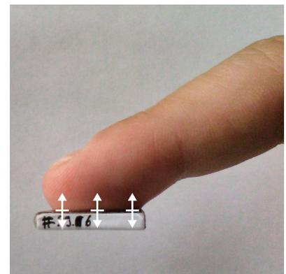
**Figure 3.** The new, strapless keystone design. Both upward *and* downward forces are now applied at the fingerpad.
