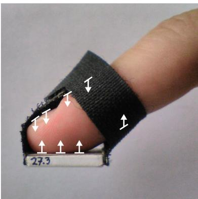
**Figure 1.** The existing, strapped keystone design. The bars with arrows indicate anatomical locations where output forces are applied. For upward forces, this is mainly at the fingerpad. For downward forces, this is mainly along the dorsal side of the fingertip.
