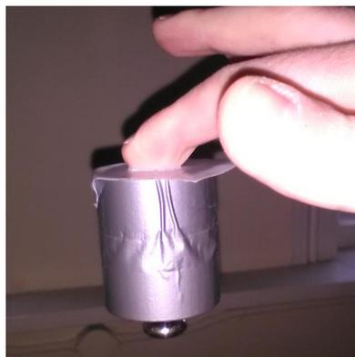
**Figure 2.** Photograph taken during preliminary testing of candidate adhesive materials. Here, measuring to-fingerpad adhesion duration under a -400 g vertical force.
